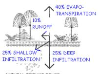
How we use land directly affects the way stormwater flows. Under undisturbed conditions, over half of precipitation infiltrates the soil and only about 10 percent runs off the surface. The natural vegetation acts like a sponge and a filter, slowing the flow and cleaning the stormwater.
